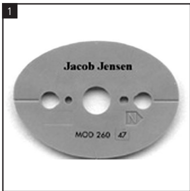
Grind the lenses in same size as Jacob Jensen former
