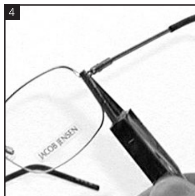
Use the Jacob Jensen plier for adjusting inclination angle
